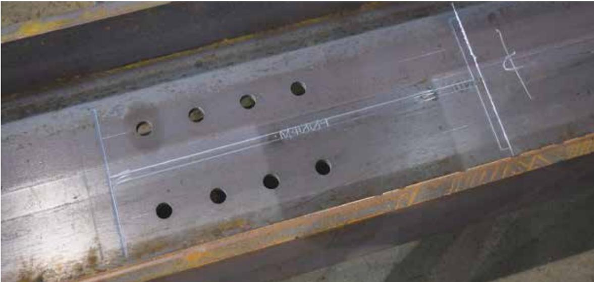
An example of the CNC layout marking system's results.
