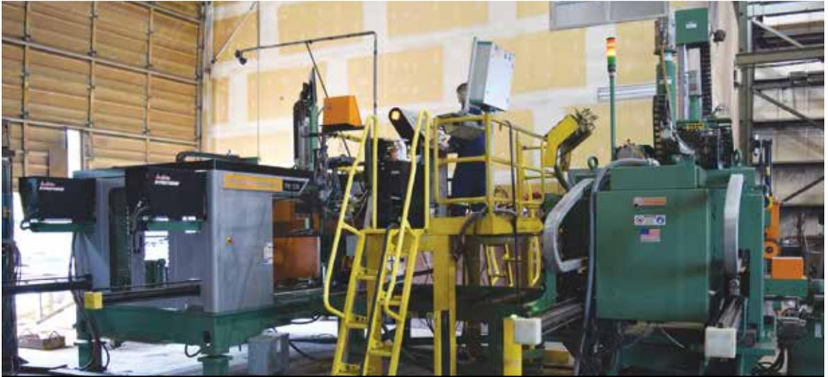
The PeddiWriter, set up in tandem with a coping machine to save space and increase productivity on the AI shop floor.
