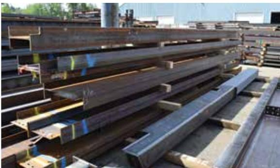
Cut and marked structural steel ready for shipping.
